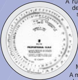
A rugged plastic dial slide rule calculator designed to calculate the new reproduction sizes at certain percentages for original artwork, copy, photographs, etc. There are four scales for reproduction size, original size, percentage of original size and number of times of reduction. Set any one of the scales and read off the values of the others. Diameter 6" (152mm), all linear size scales in inches from 0.25" to 100".
