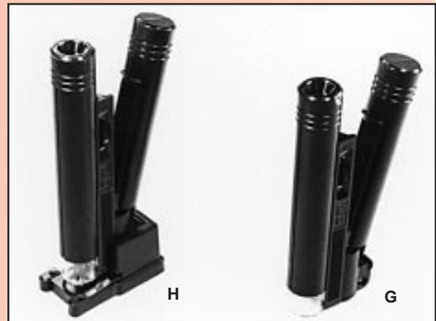
Inexpensive telescope magnifiers with a built in battery operated light source. Fine focusing is possible and the units are free standing for hands free use. Achromatic lenses are used for distortion free viewing. Two size AA batteries are required (not supplied).
