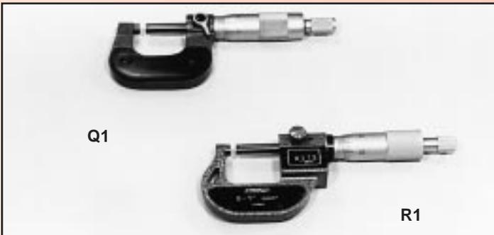
Swiss style precision micrometers with thimble ratchets for consistent measurements. Measuring faces are 0.256" in diameter and carbide tipped for long life. A positive spindle locking device is incorporated and micro fine graduations are easy to read. All models are supplied with a zero setting wrench.
