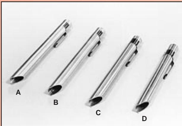
Pocket microscopes of aluminum construction. A bevelled opening gathers and focuses the light on the work surface. Lenses are of fixed focus and provide undistorted viewing. All units feature a built in measuring reticle with graduations as shown below. The microscopes are  $\frac{7}{16}$ " in diameter,  $4\frac{7}{8}$ " long and supplied with a pocket clip.
