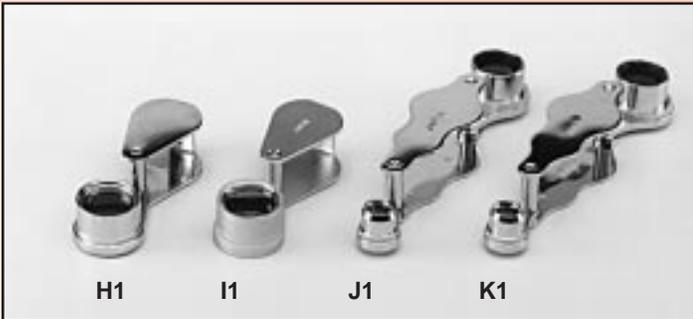
Inexpensive folding magnifiers with magnifying powers from 10x to 30x. All units feature double lens systems and metal cases with a satin finish. J1 and K1 feature two separate magnifying powers. Lenses swivel into the housings for protection and portability.
