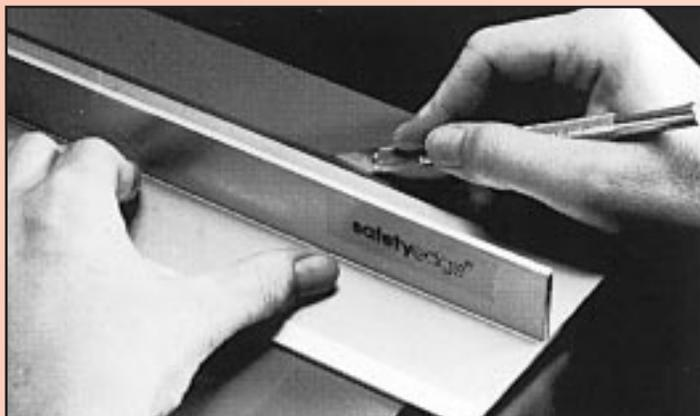
Straight edges specifically for the safe cutting of materials. The unique "T" construction protects an operator should a knife or razor blade slip or skip while material is being cut. The straight edges are manufactured from aircraft grade aluminum and feature an extra wide 3.5" wide base with an anti slip rubber covering. Used correctly these straight edges protect both the operator and artwork. A hanging hook is provided. Five sizes from 12" to 42" long are available.
