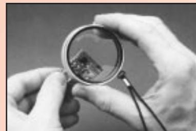
A 3x magnifier specifically designed and engineered for the repetitive observation and inspection of production parts. The low magnification and the high quality optics produce a clear, crisp, bright image and the magnifier is practical to use without eye strain. The light weight of 56gm (1.97 oz) with a convenient lens diameter of 50mm (1.97") permits tire free repetitive use. The highest quality thin optical lens is mounted in a light weight knurled aluminum barrel. A neck strap is provided.
