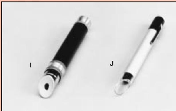
**I** A hand-held field pocket microscope of metal construction. The unit features an adjustable focus achromatic lens system with a flat field of view. The variable focusing permits magnification factors from 20x to 60x. The chrome plated base of the unit gathers and reflects light for easy viewing of an object.
