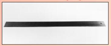
Stainless steel straight edges of good quality with a bevel on the top edge. All models are 2" wide and 0.090" thick.All stainless steel straight edges are available on special order with lifting knobs. For prices and ordering information, please contact us with details of the length of straight edge that you require and the number and placement of lifting knobs desired.
