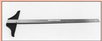
Inexpensive T-Squares of good quality with tempered stainless steel blades and aluminum heads. All models have blades measuring 1.50" x 0.060" and both edges of the underside of the blade are slightly bevelled to enable inked lines to be drawn without smudging. The head length on all models is 11.375".
