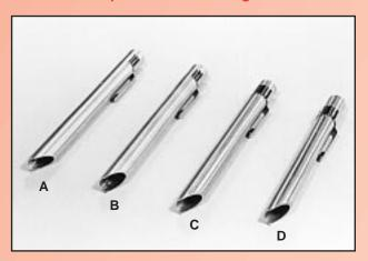
Pocket microscopes of aluminum construction. A bevelled opening gathers and focuses the light on the work surface. Lenses are of fixed focus and provide undistorted viewing. All units feature a built in measuring reticle with graduations as shown below. The microscopes are 7/16" in diameter, 47/8" long and supplied with a pocket clip.
