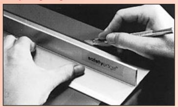
Straight edges specifically for the safe cutting of materials. The unique "T" construction protects an operator should a knife or razor blade slip or skip while material is being cut. The straight edges are manufactured from aircraft grade aluminum and feature an extra wide 3.5" wide base with an anti slip rubber covering. Used correctly these straight edges protect both the operator and artwork. A hanging hook is provided. Five sizes form 12" to 42" long are available.
