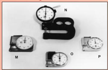
Convenient easy to read dial thickness gauges for accurately measuring the thickness of paper, card, plastic and other sheet materials. Spring loaded anvils are easily opened and measurements are read directly from the dial. All models include a small count hand to record the revolutions of the large dial hand.
