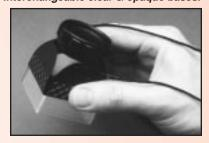
A 4x magnifier with a wide field of view of 45mm x 45mm (1.77" x 1.77"). The achromatic 27mm (1.06") diameter lens is corrected for chromatic aberration to provide a bright, clear distortion free image. The helicoid screw adjustable lens focusing mechanism is extraordinarily smooth and is the same as used in high quality photographic lenses. Interchangeable clear and opaque bases are provided as standard for regular and light table use. Supplied complete with a detachable neck
