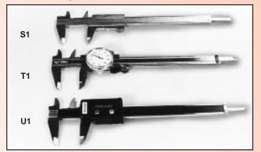
**S1** Precision vernier calipers made of hardened stainless steel with micro fine graduations. Extra long vernier ensures accuracy. Three way jaws for outside, inside and depth measurements. 0 to 6" and 0 to 150mm capacity reading in 0.001" and 0.02mm on the same unit. Measuring faces are ground and lapped. Order No.: BNS-0070A
