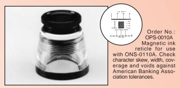
A 12x clear base comparator available with an optional 12x reticle as shown for checking the specifications of magnetic ink printing. The lens system is of the Kellner type and is 0.545" in diameter. A focusing and locking ring is incorporated. The field of view is 0.5". The glass reticle is etched on the underside to eliminate parallax errors. The comparator may be used as a regular magnifier if the reticle is not installed.
