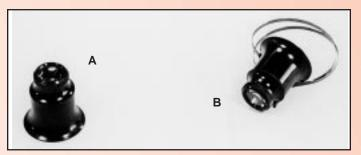
Watchmaker's and Jeweler's Loupes which are designed to be screwed into the eye or held by a metal band around the head. Each unit incorporates a two lens system with a magnifying power of 10x. One lens may be easily unscrewed and the units used with a magnifying power of 4x.
