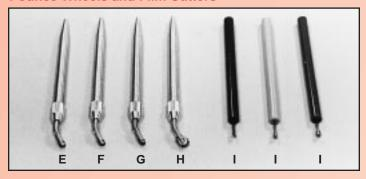
**E F G** and **H** Pounce wheels for marking and tracing patterns. The pounce wheels are designed so that they may be swiveled around circles, curves and arcs or they may be locked for straight use.
