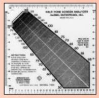
and a millimeter scale in 1/2mm. The analyzer is manufactured from durable laminated plastic for long life and measures 5" x 5" (127mm x 127mm). The analyzer is designed to measure half-tone screens from 50 to 200 and silk screen meshes from 2xx to 25xx.
