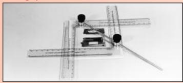
Crop and scale with ease photographs, transparencies, art, etc. Once set to the correct proportion the scaleograph enlarges or reduces automatically with no possibility of error. The scaleograph is to squares and rectangles what the compass is to circles. Units may be used on the ground glass of a camera to insure correct proportions. Two models are available.
