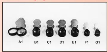
Precision folding magnifiers with a range of magnifying powers for most applications. All units have double plano convex aplantic lens systems mounted in a black lacquer metal finish housing for distortion free viewing (except A1, ONS-0210A which has a biconvex lens). Housings are made of dull chrome plated brass. Lenses swivel into the housings for protection and portability. A1 ONS-0210A has two lenses which may be used individually or together to give magnifications of 4x, 6x and 10x.
