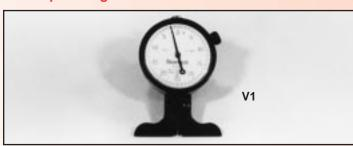
V1 A dial depth gauge with a needle point to measure depths. The knife edge base allows for precise positioning of the needle point. A light touch on the button on the top of the gauge advances the needle point until it contacts the work surface. Base length is 2.5 inches. The measuring capacity is 0.125" and the dial reads in 0.0005". The dial face is calibrated to read plus and minus from 0 to +0.025" and from 0 to -0.025".
